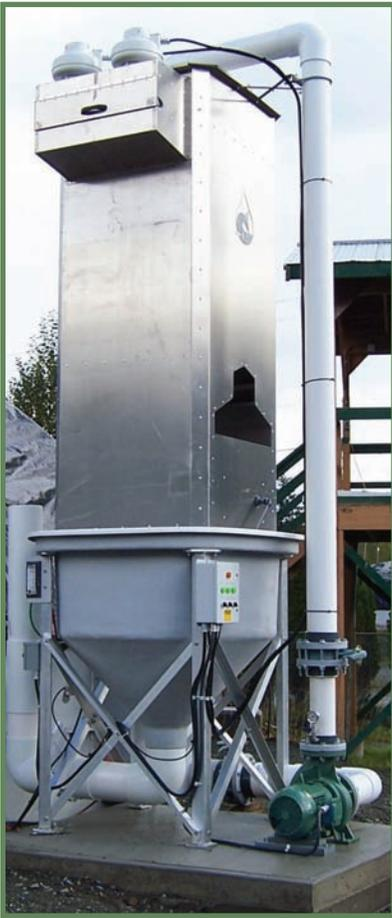
PR Aqua's OxyTower Gas Treatment Systems for culture water deliver maximum value, performance, and security to aquaculture operators. One rugged, compact unit removes carbon dioxide and oxygenates water. The cost-effective design can be used in partial reuse systems, in recirculating aquaculture systems, or in flow-through systems.
